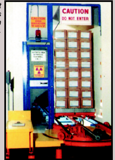
Figure 3: Product to be sterilized is conveyed into an irradiation chamber.
