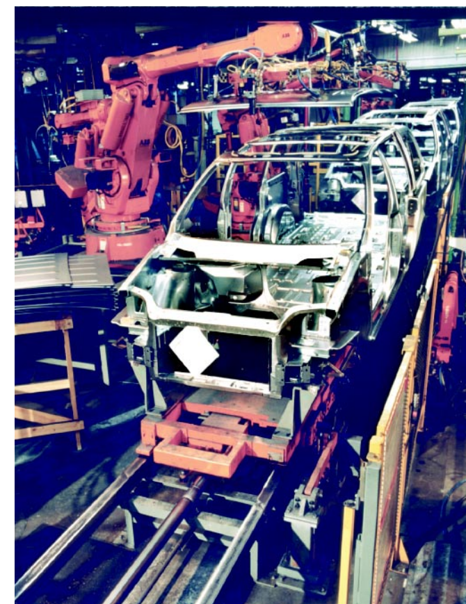
CARTRAC technology delivers reliable product flow with extreme accuracy – to within ± .005". This precise adherence to tolerance specifications has allowed companies like General Motors to improve efficiency more than 20%.
