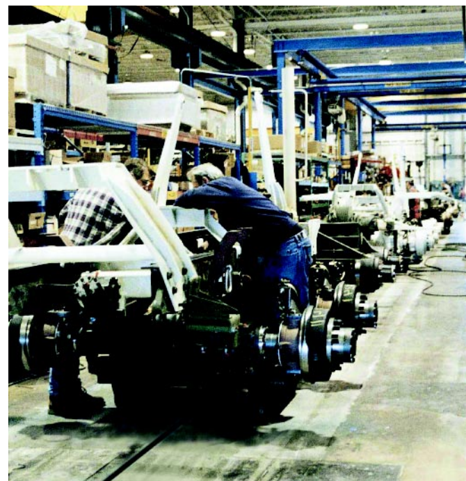
LO-TOW: One of three installations at Oshkosh Truck. This line is used to assemble axle drive train to the frame of several types of large commercial and military vehicles.
