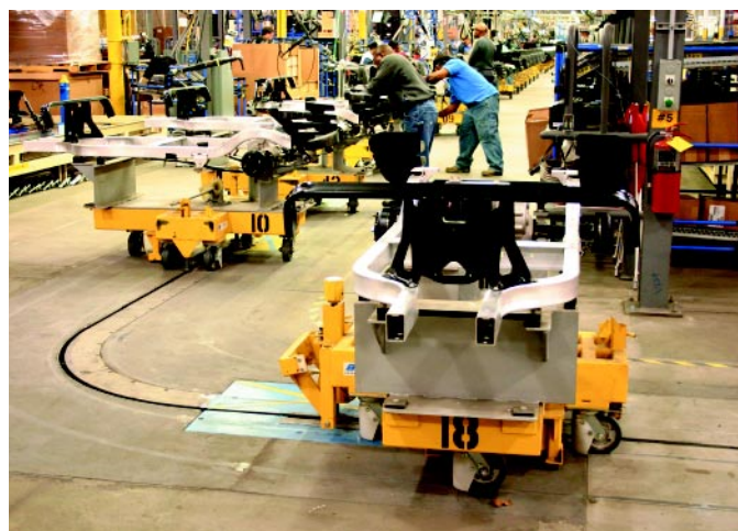
This LO-TOW towline system solution enables Club Car to custom assemble each golf car to specific customer requirements.
