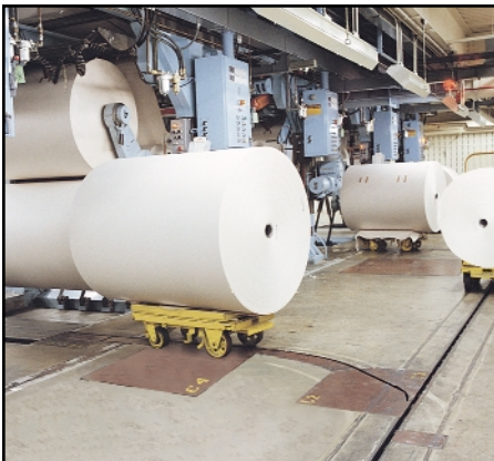
Figure 2: Rolls automatically switch into spurs for reel loading.
