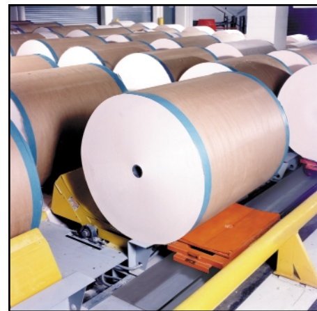
Figure 5: Stop feeder devices automatically load rolls onto dollies for transport to reels.
