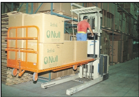
Figure 4: Carts can be designed with special devices, such as lockable fork pockets for lifting by fork trucks.
