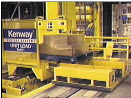
Figure 5: Precision interface can be accomplished for automatic loading and unloading by an AS/RS.
