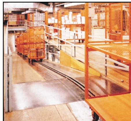
Figure 8: Lo-Tow® is perfect for moving loads up and down ramps on multi-floor buildings or on overhead bridges connecting separate buildings.
