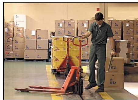
Figure 7: Pallet jacks modified to incorporate a Tow pin assembly can be efficiently used for Towline transport and off line for pallet movement.
