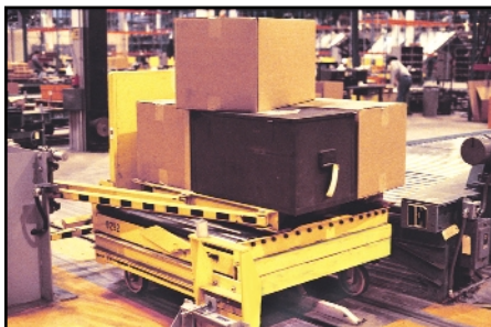
Figure 6: Pallet loads can be automatically unloaded "on-the-fly" at the correct roller conveyor line.
