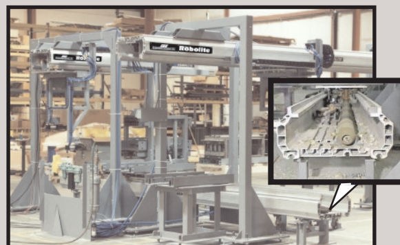
Figure 6: Both floor mounted and inverted over-head Robolite (extruded aluminum version) are combined in this installation for handling a corrosive polymer material. (See insert.)
